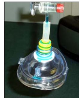
Study 2b: Coloured water dripped from burette onto filter. Volume measured to when leakage occurred from filter
