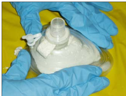
Study 2a: Builders foam introduced whilst mask held flat on surface to check for areas of leakage (valve)
